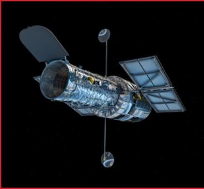
**Dimensions:** Length: 13.2 metres, diameter: 4.2 metres. In addition two solar panels each of which are 2.45 x 7.56 metres.
